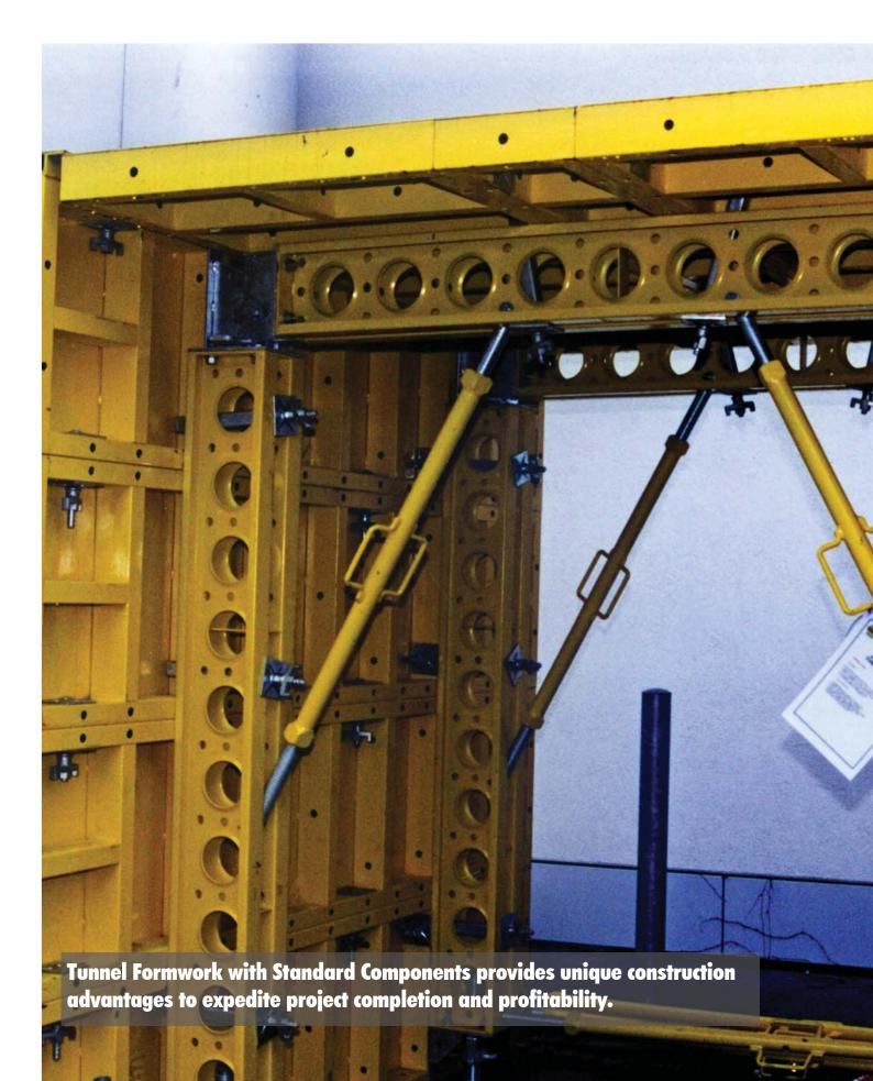
Tunnel form is a formwork system that allows construction of cellular walls and slabs in one operation on a daily cycle. It combines the speed, quality and accuracy of offsite production with the flexibility and economy of on-site construction and is recognised as a modern method of construction. The result is a cellular reinforced concrete structure, the surfaces of which are of sufficiently high quality to require only minimal finishing for direct decoration.
